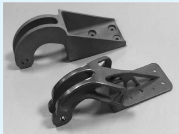
FIGURE 15.6 Top: Conventional Hinge; Bottom: Same Hinge, Half the Weight Using 3D Printing Technology
