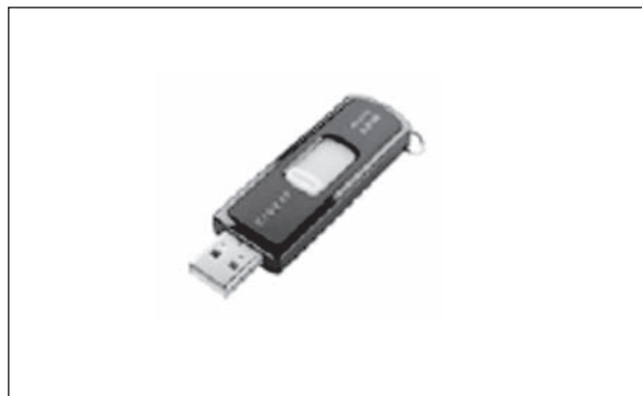
FIGURE 2-13 This Flash memory from San Disk plugs into a standard USB microcomputer connector. It can write data at 13 mb per second, read data at 15 mb per second, and store up to 4 gigabytes of data.
