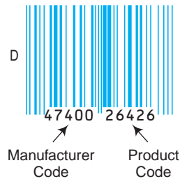
FIGURE 2-3 An example of the universal product code (UPC), which is often preprinted on the labels of retail products for merchandise identification and computerized checkout.
